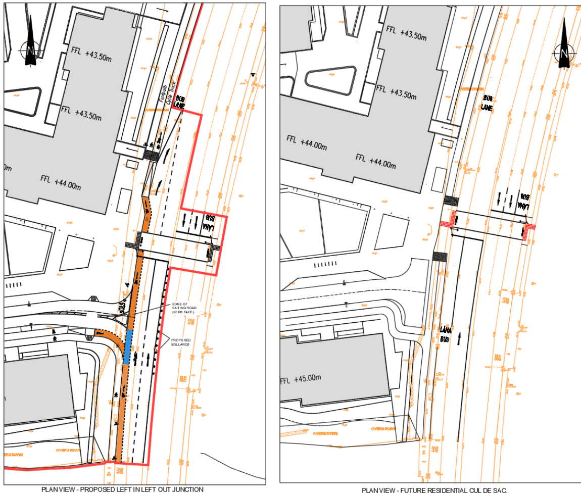
Figure 5 – Left in/Left Out – Temporary Arrangement (left hand image) and Future Permanent Arrangement (Right hand image)
